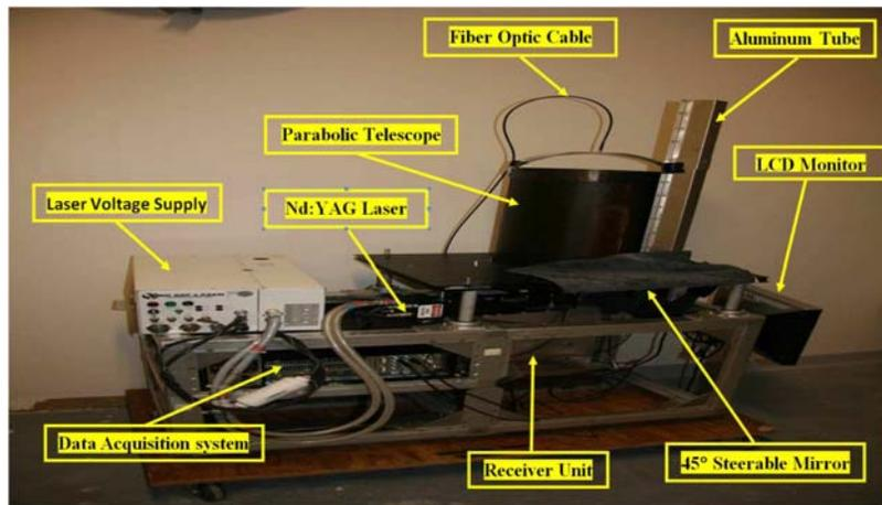
Figure 2. Lidar in Vision Lab at Old Dominion University
